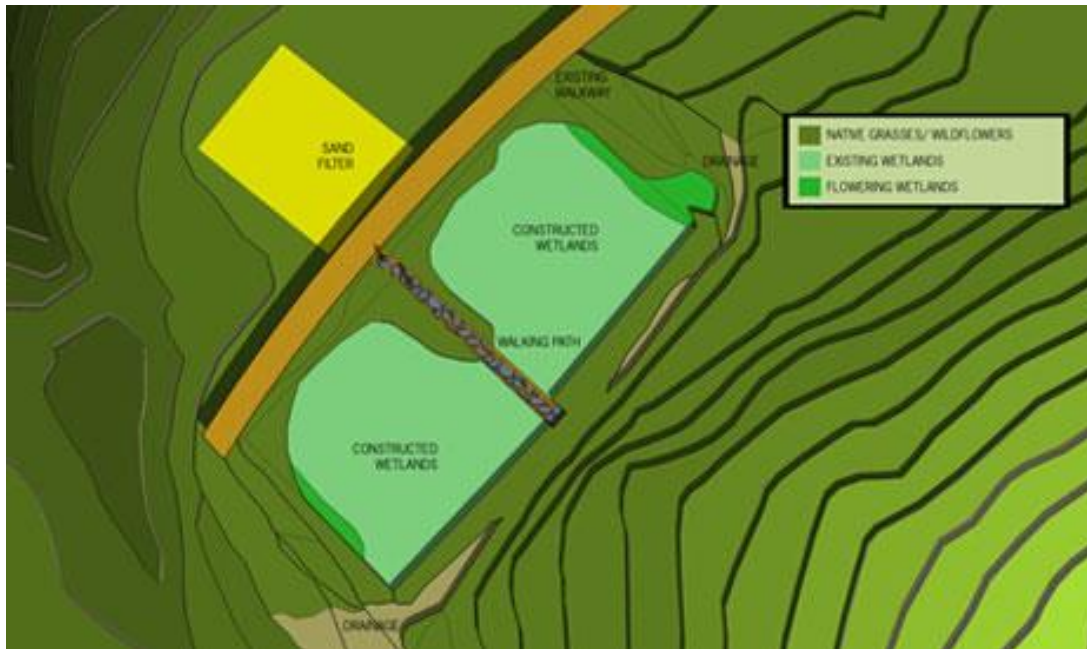
Figure 4.43 Plan View of Natural Wastewater Treatment Plant
